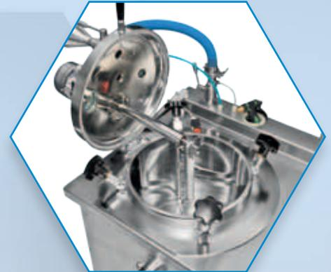
Removable mixing blades with wall's scrapers.
